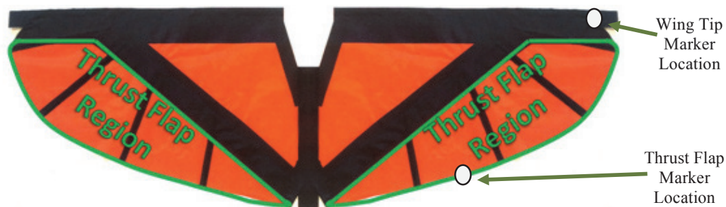
Figure 19. Wing planform showing the thrust flap region and the locations of the wing tip and thrust flap markers.
